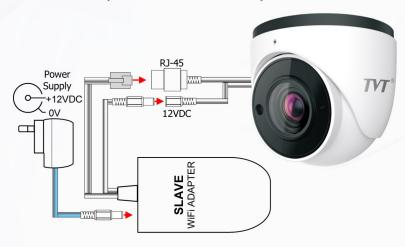
The slave wifi adapter can be placed in-line with a power supply for an IP Camera (as shown in the above diagram)
