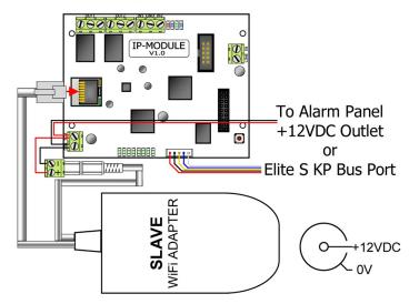
The slave wifi adapter can be powered directly from the alarm system or from the IP-MODULE's pass through terminal (as shown in the above diagram)
